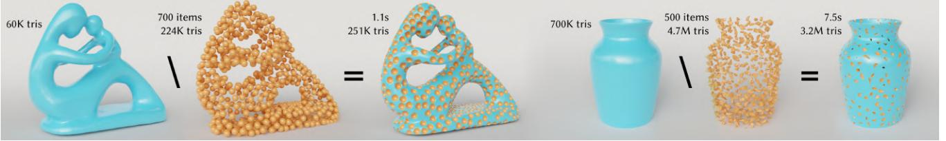
Fig. 9. Our method scales optimally to variadic Booleans involving hundreds of shapes. We executed the operations in the figure in two different ways: passing in input each decorative element separately, and merging all decorative elements into a single input mesh. In both cases the running time was the same, thus no computational overhead was introduced for the increased number of input shapes.
