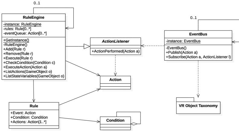
Fig. 2. Class diagram for the ECA rule engine.
